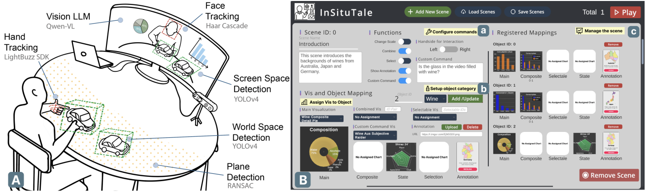
Figure 4: Presentation and Authoring Modes: InSituTale consists of presentation and authoring mode. (A) In presentation mode, the presenter interacts with visualizations in real time using physical objects and hand gestures, tracked by a depth camera placed in front of them. A live video stream is displayed locally for monitoring. (B) In authoring mode, the presenter configures physical objects, commands, and visualizations to be used during the presentation.
